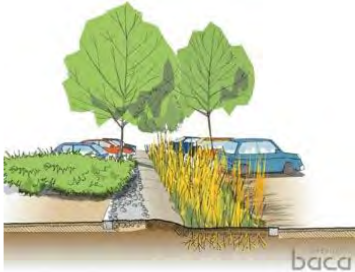
Figure 15 Vegetated Filter Strip
