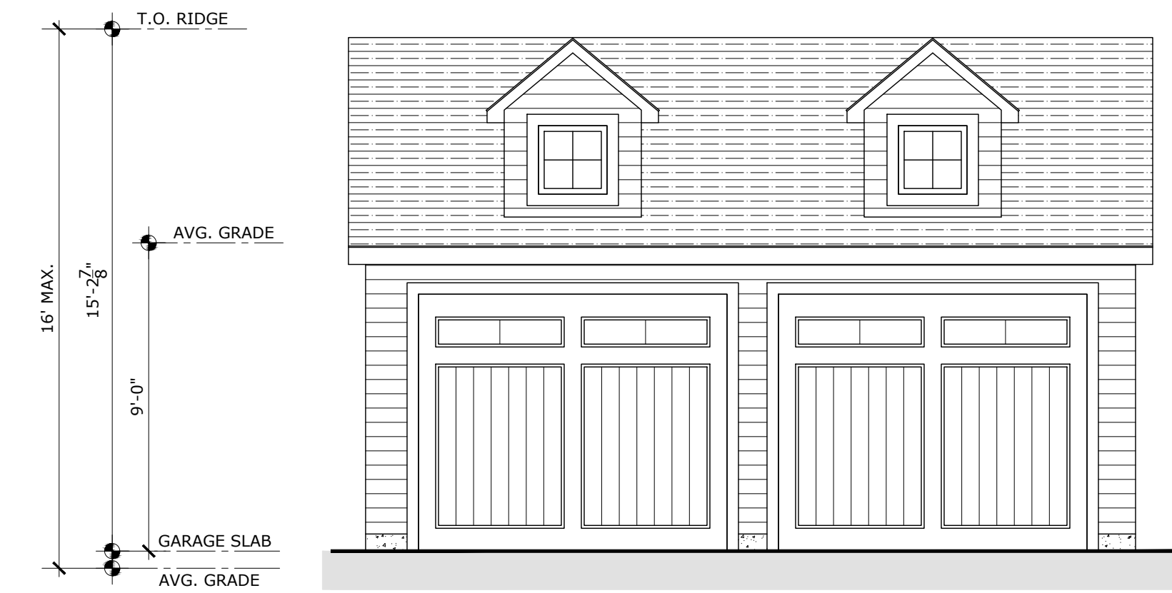
4 A2 GARAGE FRONT ELEVATION 1/4" = 1'-0"
